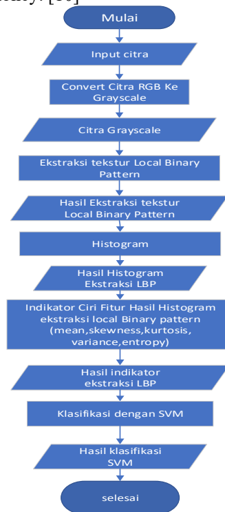
Figure 3. LBP And SVM Algorithm Flowchart
